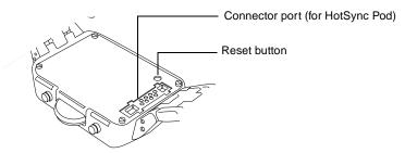
**HotSync Pod connector port.** Lets you connect the cable from the HotSync Pod to recharge the watch and perform HotSync® operations.
