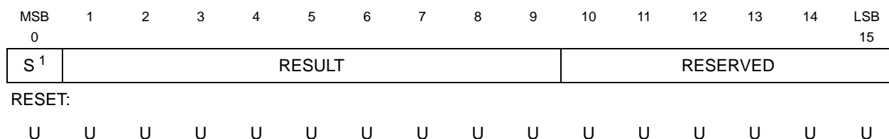
Figure 13-19. LJSRR — Left Justified, Signed Result Format 0x30 4B00 – 0x03 4B7F, 0x30 4F00 – 0x03 4F7F
