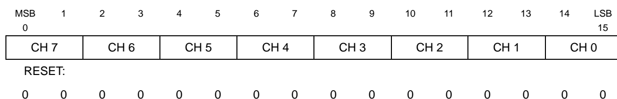
Figure 18-19. CPR1 — Channel Priority Register 1
