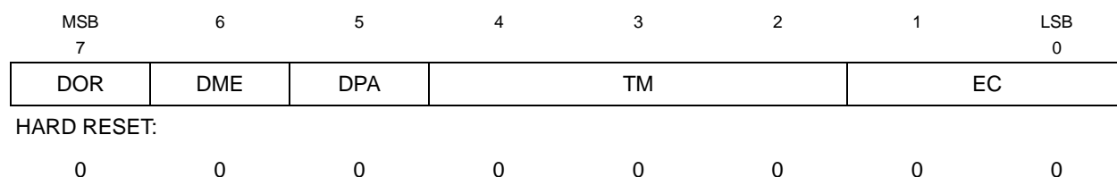
Figure 23-4. READI_DC — READI Development Control (DC) Register0x0A
