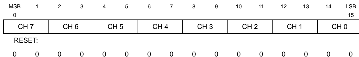
Figure 18-15. HSQR1 — Host Sequence Register 1
