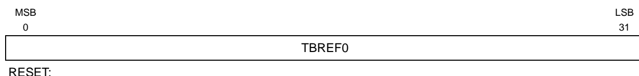
Figure 6-32. TBREF0—Time Base Reference Register 0 0x2F C204
