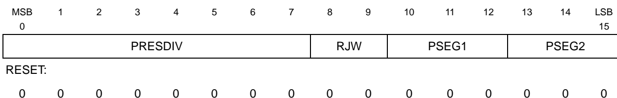
Figure 16-13. CANCTRL2 — Control Register 2 0x30 7088 0x30 7488 0x30 7888
