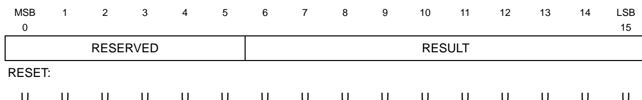
Figure 13-18. RJURR — Right Justified, Unsigned Result Format 0x30 4A80 – 0x30 4AFF, 0x30 4E80 – 0x30 4EFF
