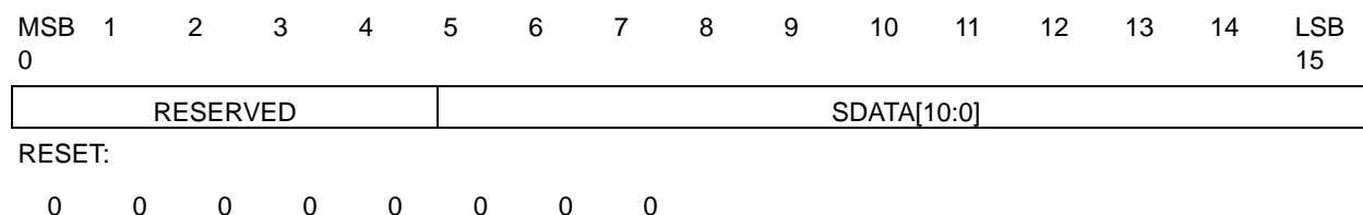
Figure 15-23. SDATA— Symbol Timing Data Register 0x30 008A
