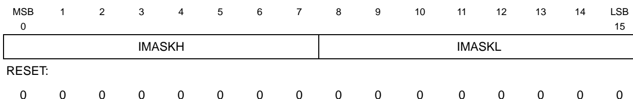
Figure 16-17. IMASK — Interrupt Mask Register 0x30 70A2 0x30 74A2 0x30 78A2
