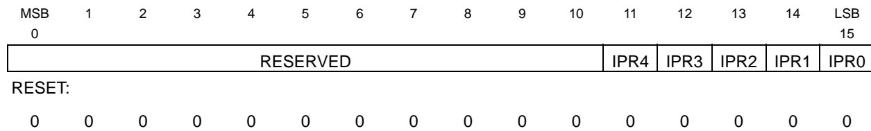
Figure 15-18. IPR — Interrupt Pending Register 0x30 0084
